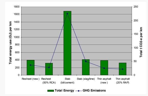
Cement substitution can reduce emissions by 70% Recycled aggregates substitution - by 25 - 40%
